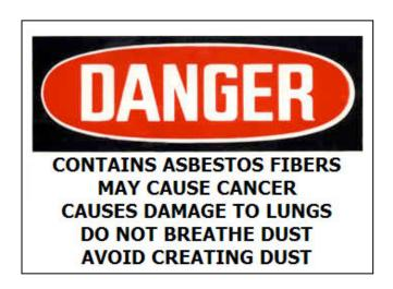
Asbestos waste shall be properly labeled with a 'Danger – Asbestos' label, DOT Class 9 Special Waste label and generator tag.
