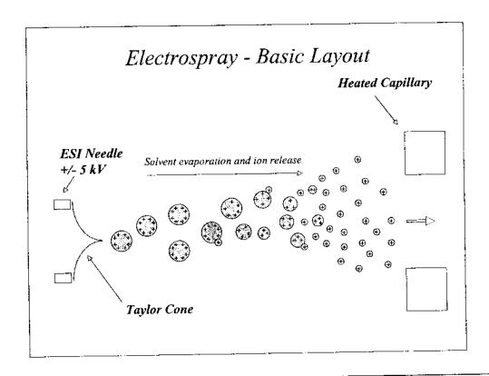
The first step of ion formation in electrospray is droplet fragmentation at the needle tip. The interaction of the high voltage and sheath gas causes the solution flow to form a "Taylor Cone." This emits very small charged droplets. The droplets are enriched with analyte ions of the same polarity as that applied to the ESI nozzle, since those charges were repelled from the needle and opposite charges were grounded by the needle.
