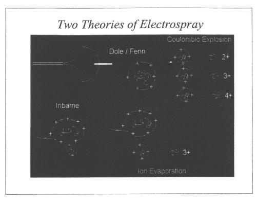
There are two competing theories as to what is occurring during the desolvation of solvent flow between the probe and heated capillary. Both agree that very small droplets are broken off of the main flow at the Taylor Cone. Then, the process by which desolvation occurs differ for each theory.
